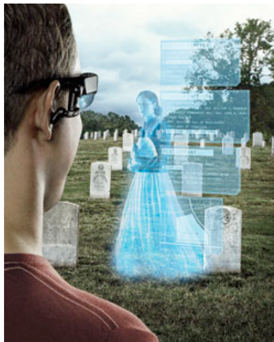
An example of the magic lens metaphor. The user, who is wearing a head-mounted display, sees a virtual woman in the real-world graveyard.
